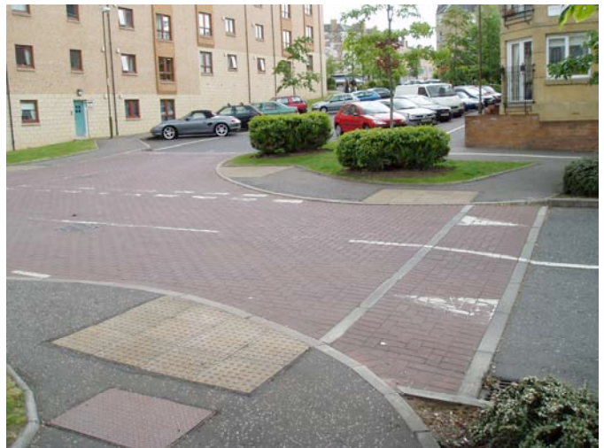
Raised platforms, narrowed road or signs that mark the beginning of residential streets.
